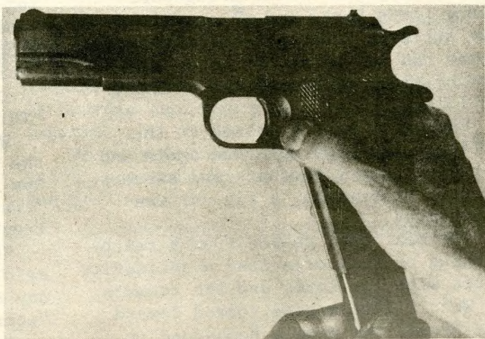
Press magazine catch with right thumb and, at same time, withdraw magazine from receiver. Pull slide to rear and look in chamber to see that gun is not loaded. Close slide and pull trigger so hammer is down
